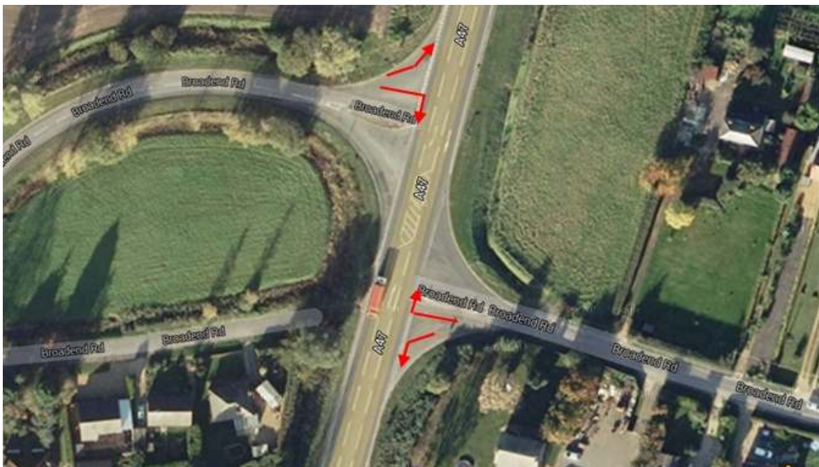
Figure 2.6: Turning Movements used to Calculate Average Delay at Broadend Road Junction
